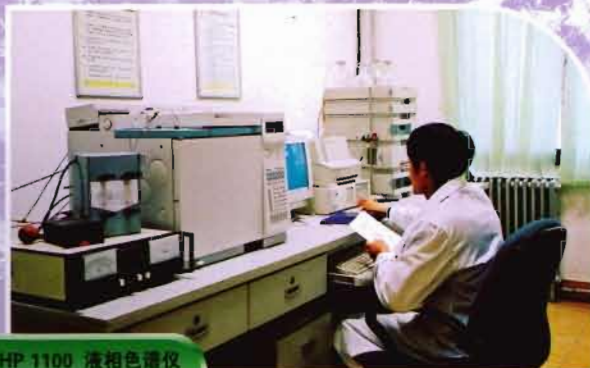
HP-6890 气相色谱仪 HP 1100 液相色谱仪 HP-6890 Gas Chromatography HP 1100 Liquid Chromatography
